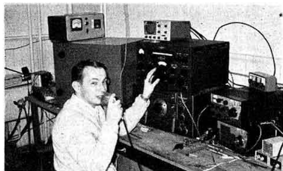
Pete, K2RBT/6, is a keen 3.5 MHz addict and has been heard and worked on that band from Europe. His QTH is 500 ft asl and his equipment includes a TR4, RV4, 75A4, and a 4CX1000 linear—not to mention a 2 element \frac{1}{2} wave vertical beam.
